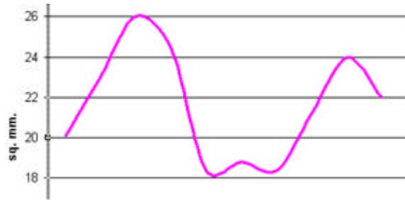
**Picture 10. Variation of the total contact area on rotating WN gears.**
