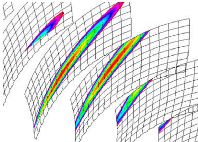
Picture 9. Visualization of the tooth contact on all the teeth in the mesh on involute gear.
