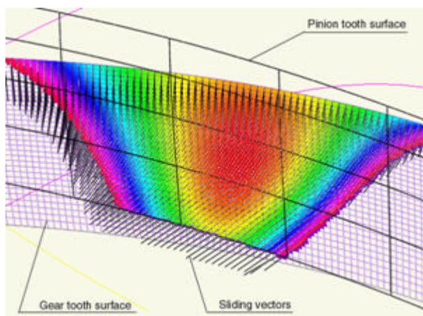
Picture 3. 3-dimensional simulation of WN contact.
