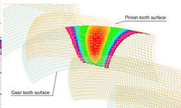
Picture 4. High resolution of WN mesh simulation.
