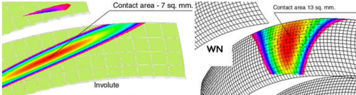
Picture 7. Comparison of the contact area for similar size WN and involute gears.
