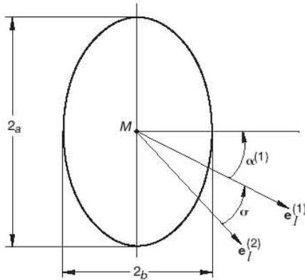
Picture 12. Elliptical form of WN tooth contact reported by NASA. Faydor L. Litvin, Pin-Hao Feng, and Sergei A. Lagutin "Computerized Generation and Simulation of Meshing and Contact of New Type of Novikov-Wildhaber Helical Gears" NASA CR-2000-209415 ARL-CR-428, October 2000, page 15.
