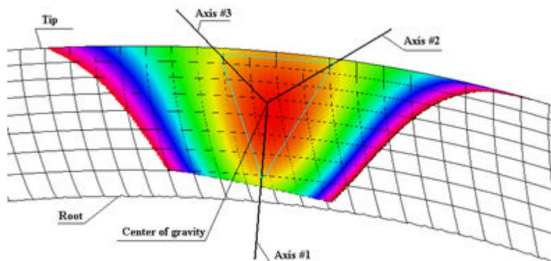
Picture 14. Three axis of the contact pattern discovered by the author on WN gears.
