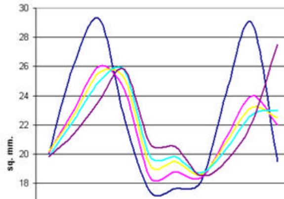
**Picture 11. Total contact area of WN gear for different helix angle.**
