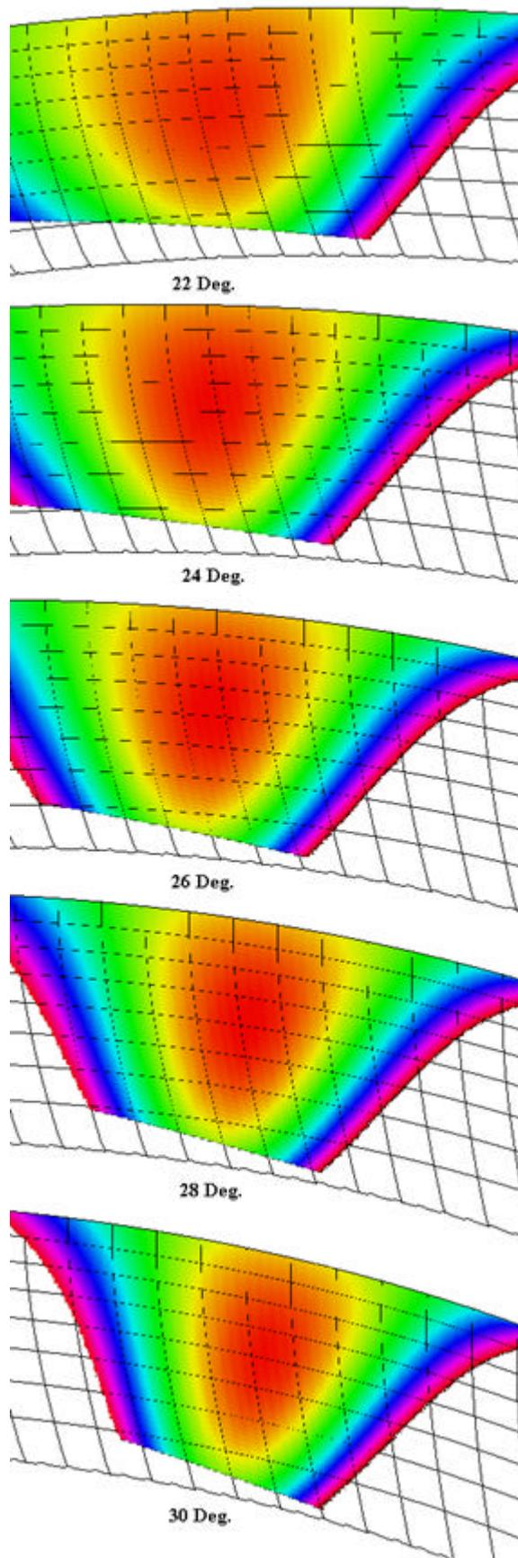
Picture 17. WN contact for different helix angle.
