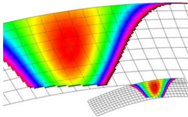
Picture 13. Correct 3-d visualization of WN tooth contact.
