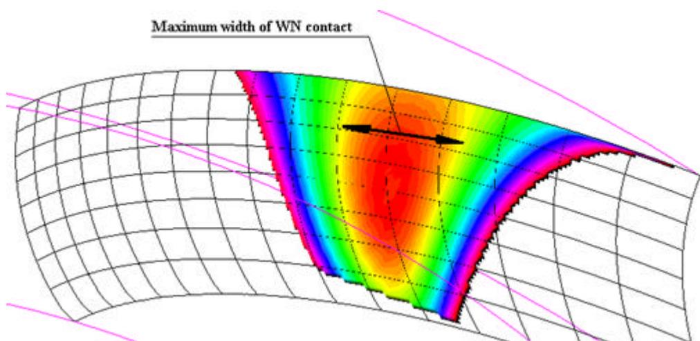
Picture 16. Off set of the maximum width of the contact.
