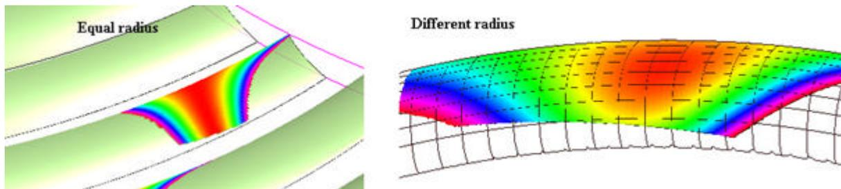
Picture 15. Different contact forms for different radiuses of WN profiles.
