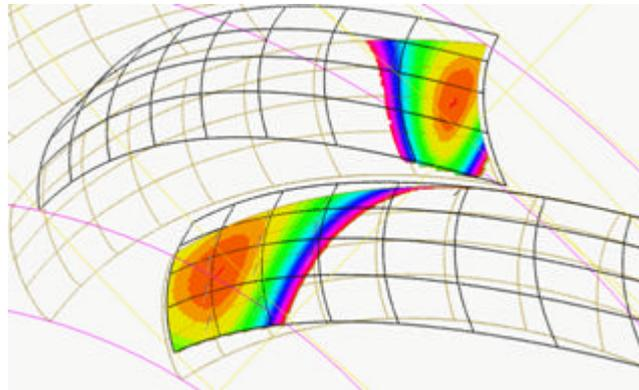
Picture 8. Visualization of the tooth contact on all the teeth in the mesh on WN gear.
